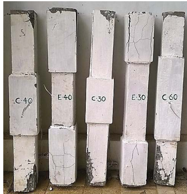
Fig. 6. Failure patterns of partially jacketed specimens
