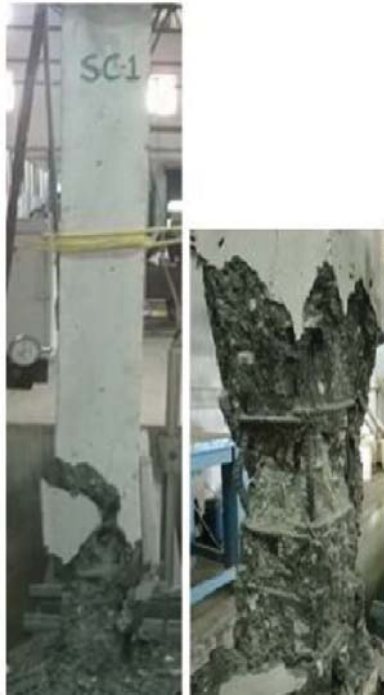
Fig. 4. Failure patterns of square control specimen
